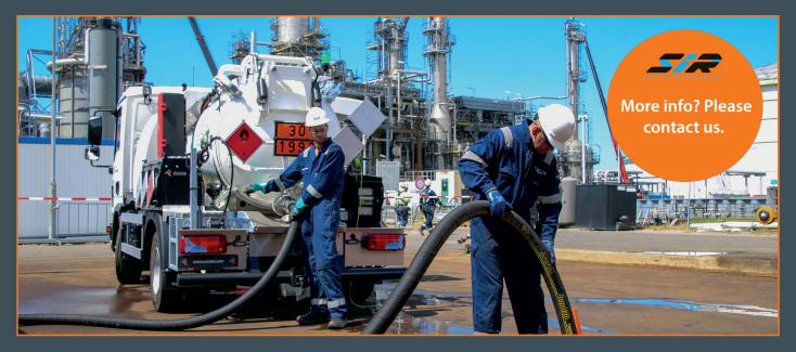
Using the ROM VAC - ADR vacuum unit, you can suck up and transport liquid substances and sludge. With the addition of ADR, the machine is also suitable for hazardous substances, such as combustible substances and oils. The compact design is ideal for places that are difficult to reach, such as tight driveways and oil clean up operations. In addition to the very capable basic version, there is a wide choice of options, including SIR certification.
