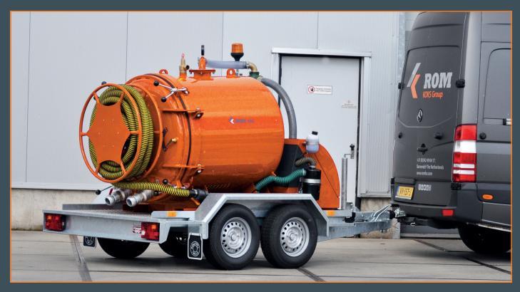
The ROM VAC pick-up units are intended for the simple emptying of grease traps, septic tanks and surface water drains. The compact design is ideal for places with difficult access such as shopping centres and schoolyards. The vacuum units are also suited for suctioning the excess water after flooding problems. The installations are available in 1200 and 1750 liter tanks and offer the perfect to expand your activities.
