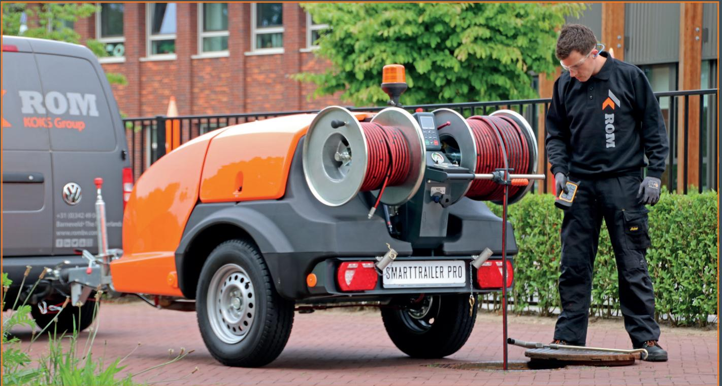
The new ROM SmartTrailer PRO sewer jetting trailer: packed with smart solutions based on over 40 years of experience. Perfect for the unblocking and cleaning of lateral lines and main lines in the sanitary sewer system up to Ø400mm. You can go for a petrol or a diesel engine, a cleaning pressure of up to max. 160 bar and a water capacity of up to max. 60 l/min.
