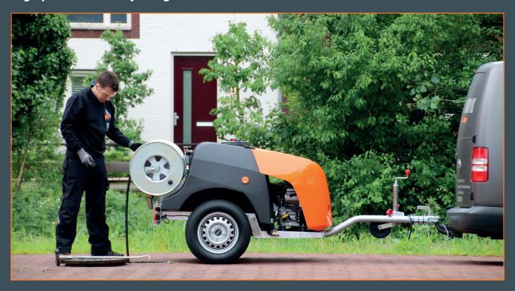
The ROM SmartTrailer sewer jetting trailer is suitable for the unblocking and cleaning of lateral lines and main lines in the sanitary system up to Ø300mm. The machine can also be employed for facade, surface and drain cleaning. The trailer can even be used for light graffiti removal. The perfect solution for sewer cleaners, plumbers and municipalities.
