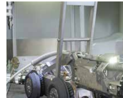
Lowering/lifting hook For easy insertion of the crawlers into the sewer.
