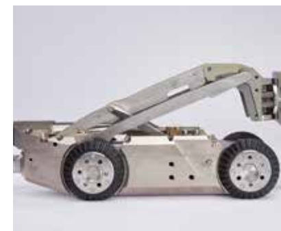
Electrical lifting gear Continuous camera positioning from 150 mm.
