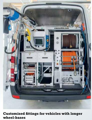
With increased space requirements – such as for additional high-pressure jetting units or pressure test units - we rely on vehicles with longer wheelbases. We also offer four-wheel drive solutions or box trucks.
